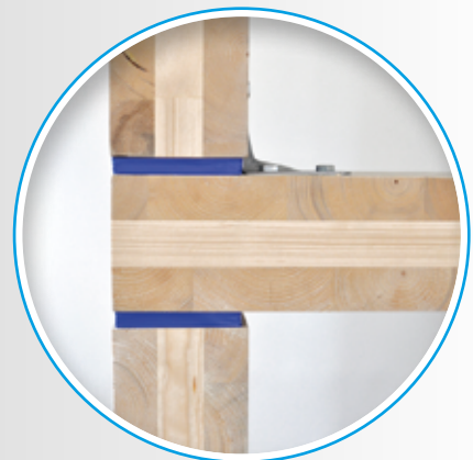
Tested build-up with angle joints and screws
